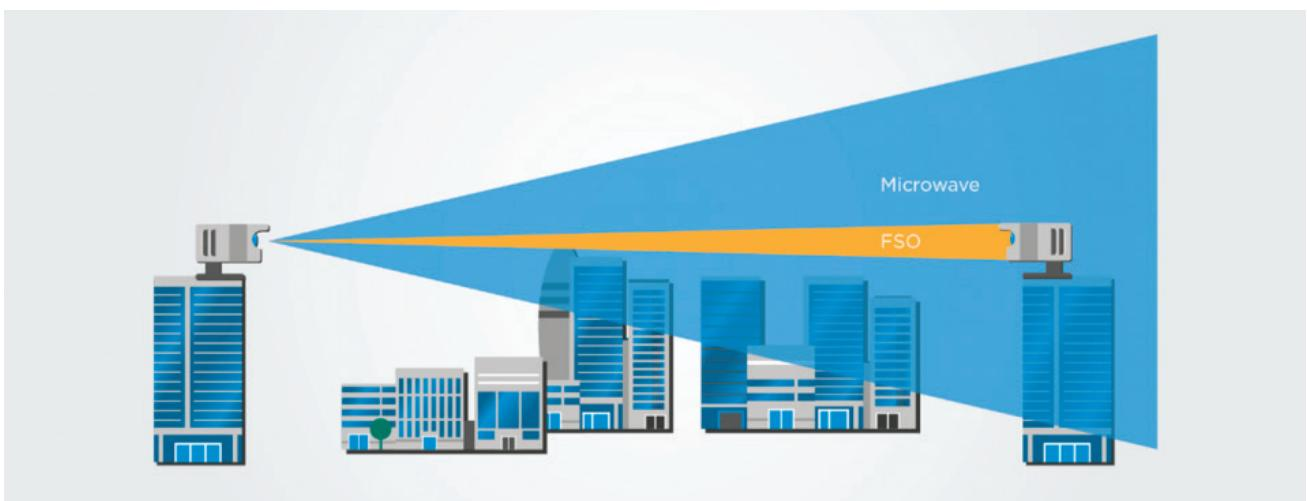
*Geometry of an FSO system vs. a microwave link. The microwave link has a much wider spread than FSO, which makes eavesdropping and jamming easier.*
